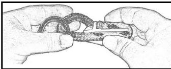
Step 3 Follow the arrow up to #2 across to #3. Follow arrow down to channel #4. If you attached hardware in Step 1 now slide fixed hardware onto the loop. Now pull line across to #5. Pull on line to snug while holding onto the lines along the grooves with three fingers. Take line up to #6
