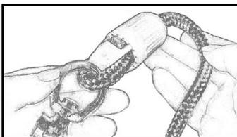
Step 5 Screw together until the nut bottoms on the core, stop approximately every three turns and pull the line tight, this keeps the line from bunching together under the nut. See the done illustration, note line at inspection port.
