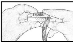
Step 2 Hold Core with groove 1-2, 3-4 facing towards you in one hand and in opposite hand hold the bitter end of line with the nut already attached. Find groove 1-2 and place the bitter end of the rope at the stop located next to the #1
