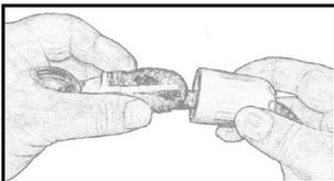
Step 4 Place Nut on core still holding the line securely with three fingers rotate 2 times and stretch the line tight into the grooves
