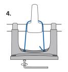
4. **Fix cable on one side** by tightening the locking bolt. Pull the other end downwards firmly and tighten the bolt. Take care to have both key bolts firmly tightened (5Nm).
