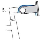
5. **Push holder downwards** until it is stopped by the cable and tighten the 4 screws (1Nm).
