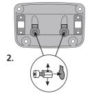
2. Insert the two locking nipples.
