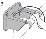
3. **Feed cable** from under front structure of handlebar into the locking nipples incorporated at the backside of the holder.
